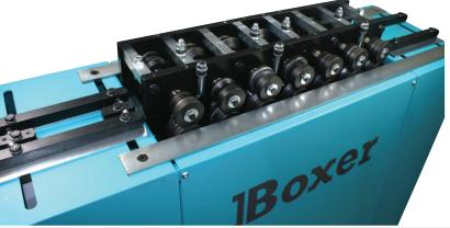
The Pittsburgh rolls are fitted between sideplates, with the option to fit 1 of 10 CNC machined roll sets to the outboard extension shafts (see back page). Our 16s Pittsburgh roll set incorporates automatic material gauge compensation, to ensure tight definition of the seam throughout the gauge range.
