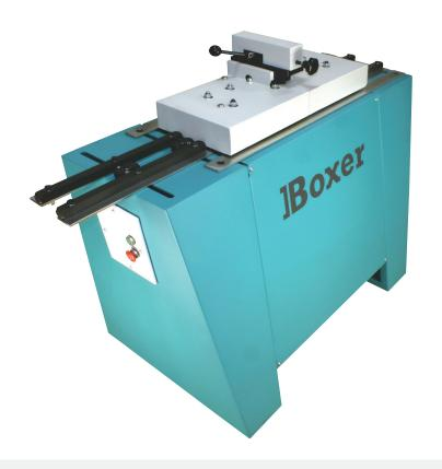
The Boxer flanging attachment can be fitted to any of the Boxer standard lockformers and is capable of forming up to 10mm flanges on products between 0.4 and 1mm thick. An option to produce a completely flanged disc is available, utilising a pivoting front roll.
