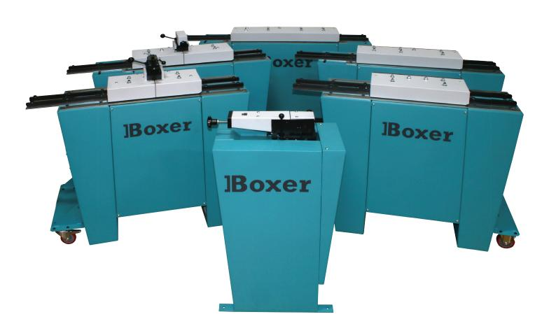
The lockforming machines possess between 5 and 12 pairs of rolls, mounted at 102mm horizontal and 63mm vertical centres and are driven at a throughput speed of 10m/min.
