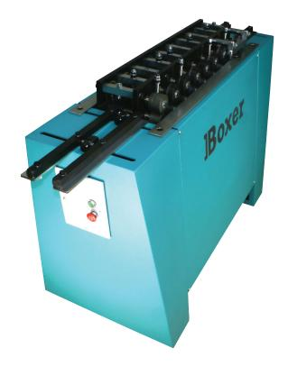
This system is used as a simple method to join between 0.6mm and 1.2mm sheet metal at right angles and is designed to lock rigidly together, without the need for a post seaming operation. See back page.
